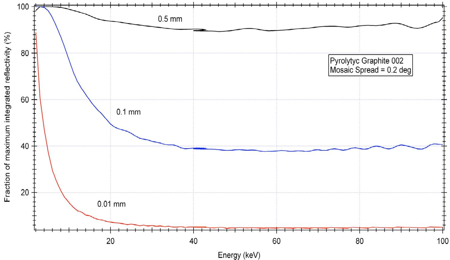
Trade off on the reflection/thickness behavior has to be considered. Thinner crystals allow us to **reduce the cost** and to **better fit the shape** of figured double-curvature mirrors!
