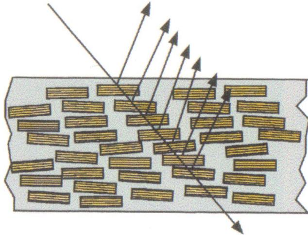
Bragg diffraction of a laminar monochromatic beam with an *ideally imperfect crystal* (perfect mosaic)
