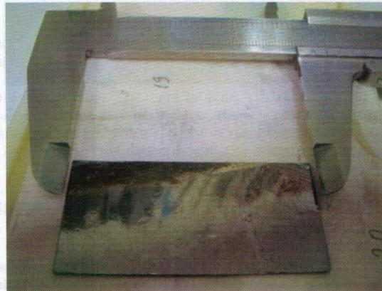
Figure 5.4: The sample of HOPG crystal by *Advanced Ceramics*,  $6 \times 2 \times 0.2$  cm<sup>3</sup>.
