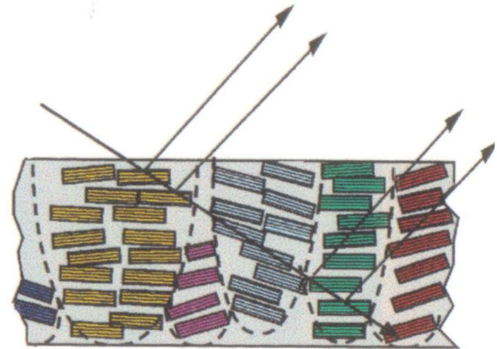
Bragg diffraction of a laminar monochromatic beam with an mosaic crystal containing macrostructures
