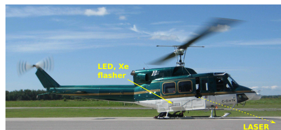
Figure 4: The light sources were mounted on a Bell 212 helicopter. This dual turbine model was used because it satisfied various rules for night flight in Canada.
