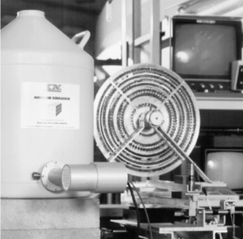
Fig. 1 The gamma-ray lens and the 3x3 Germanium matrix during the ground based system tests at ANL. When operating in the focal spot of the lens, the Ge detector is located 10-20 m behind the lens.
