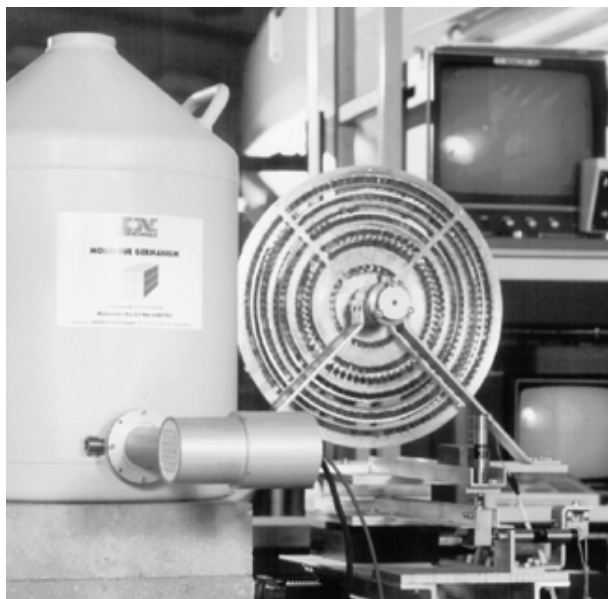
Fig. 1 The prototype gamma-ray lens and the 3x3 Germanium matrix during the ground based system tests at ANL. When operating in the focal spot of the lens, the Ge detector was located 10-20 m behind the lens.
