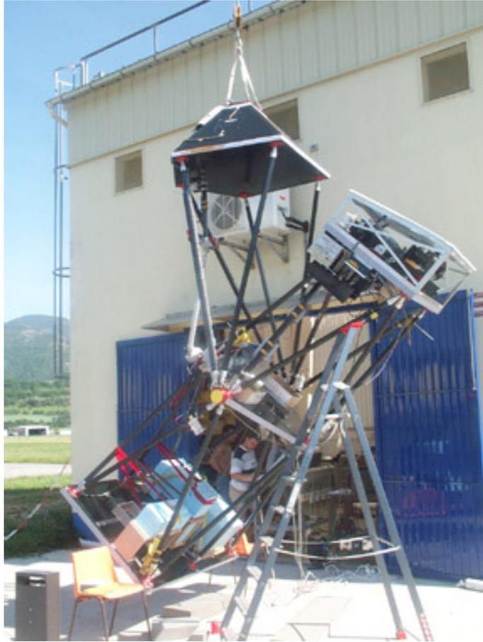
**Figure 2.** CLAIRE during pointing tests at the launch site.
