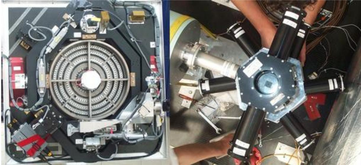
**Figure 3.** Left : CLAIRE's  $\gamma$ -ray lens (diameter 45 cm on the gimbal mount of the fine pointing system. Right : The 3x3 HP-Ge matrix surrounded by the anti-coincidence shield.
