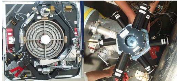
Figure 5. Left : CLAIRe's \gamma -ray lens (diameter 45 cm on the gimbal mount of the fine pointing system). Right : The 3 \times 3 HP-Ge matrix surrounded by the anti-coincidence shield.
