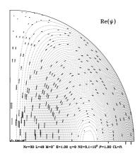
Fig. 2. Meridional flow of the convection cell that appears at the threshold of instability in a sphere when the fluid is heated by a uniform distribution of heat sources.
