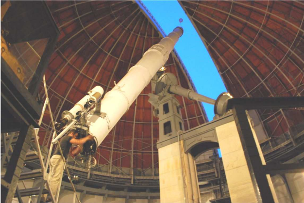
Fig 1.4-1: 200 mm aperture, 18-meter focal length Fresnel primary array placed at the front end of a 19-meter refractor tube for validation on sky sources. (696 Fresnel zones, ~250 000 subapertures).
