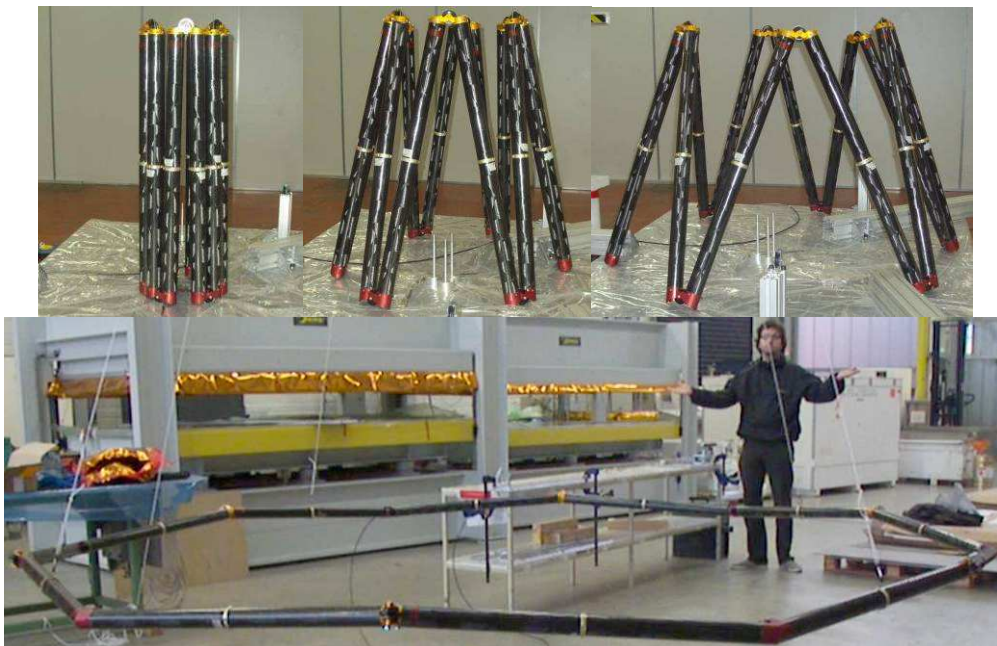
Fig 5.10-1: photographs of structure prototype (mass: 10.3 kg) folding and unfolding.
