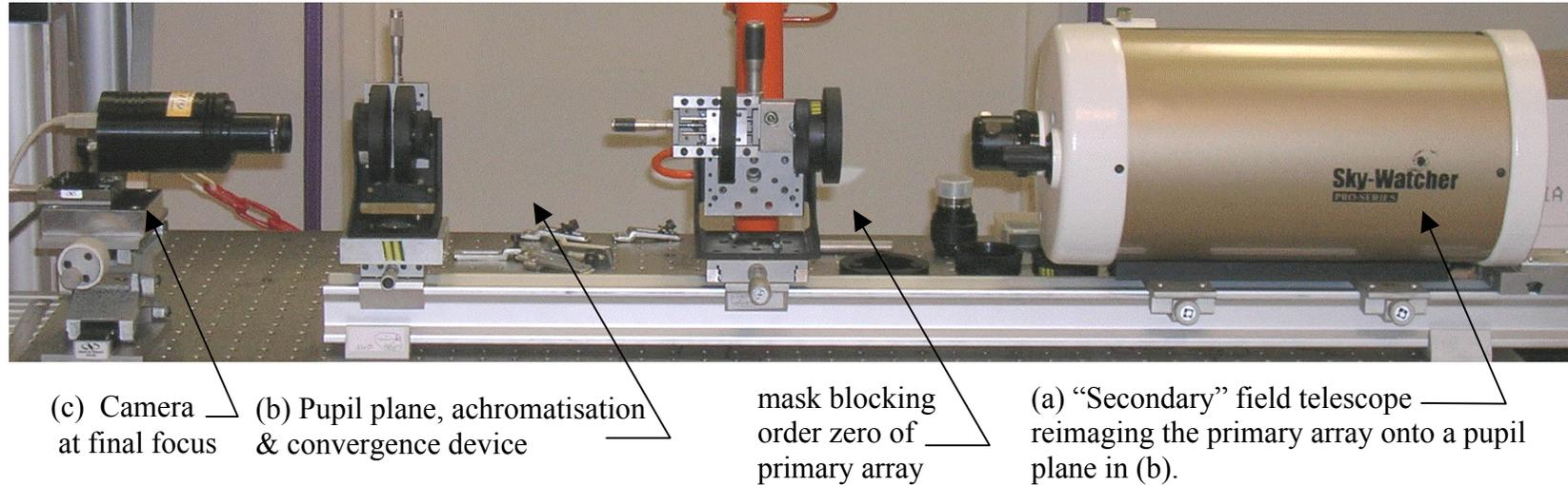
Fig. 6: Field optics and focal instrumentation
