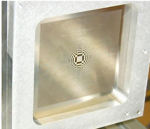
Fig. 3: 80 mm square primary array carved into a thin 80  $\mu\text{m}$  stainless steel foil, used for optical tests.
