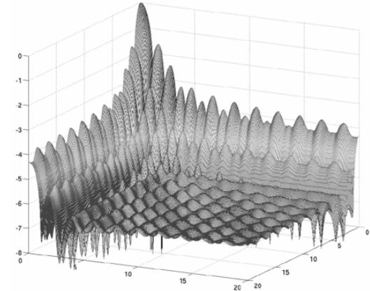
Fig. 5: Numerically computed PSF (quarter field) of an apodized 800 zone Fresnel array of size B, showing the central peak and two of the four orthogonal spikes. The dynamic range reaches  $10^7$  in most of the field.
