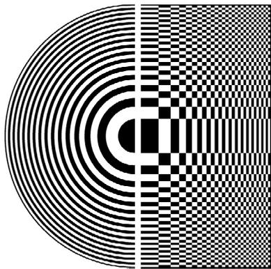
Fig. 1: Circular (Soret) zone plate & example of orthogonal Fresnel array, 15 Fresnel zones (half sides).
