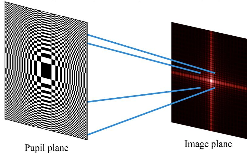
Fig. 2: Image of a point source, low levels enhanced: power 1/4 viewing. Point Spread Function computed by Fresnel Transform.
