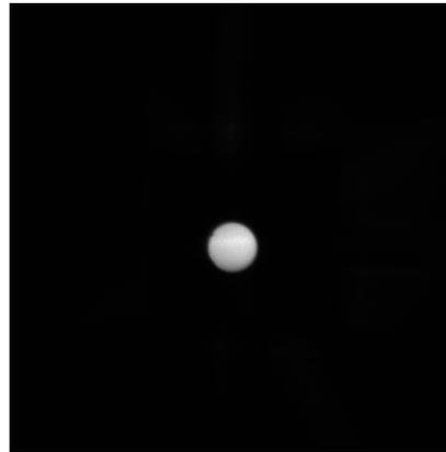
Fig. 4: a 32 arc second disk, imaged by the 80 mm achromatized test array. The disc is a 200  $\mu\text{m}$  pinhole illuminated in broad band by a halogen lamp and collimated by a 1270 mm focal length mirror. The detector is a SXV-H9 ccd camera sensitive from  $\lambda = 0.5$  to 1.1  $\mu\text{m}$ . There is no detectable chromatic aberration. The white horizontal strip in the disc is due to the lamp filament.
