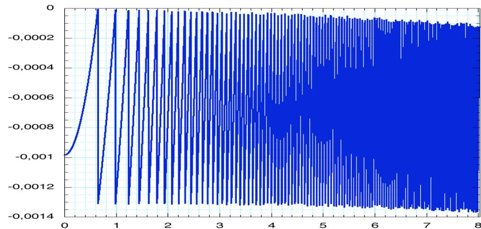
Half profile of the blazed fused silica diffractive lens.
