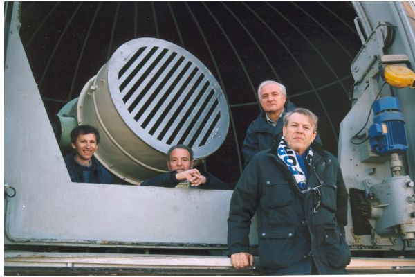
FIGURE 7. Grating mask mounted on the Zeiss telescope for scale absolute calibration, and some members of the PISCO team (from left to right: J.-L. Prieur, M. Scardia, R. Valtolina, L. Pansecchi).
