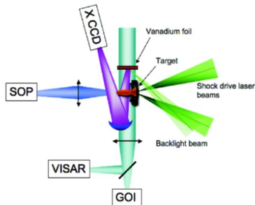
Rear-side illumination of target  $\rightarrow$  easier to place an ambient medium
