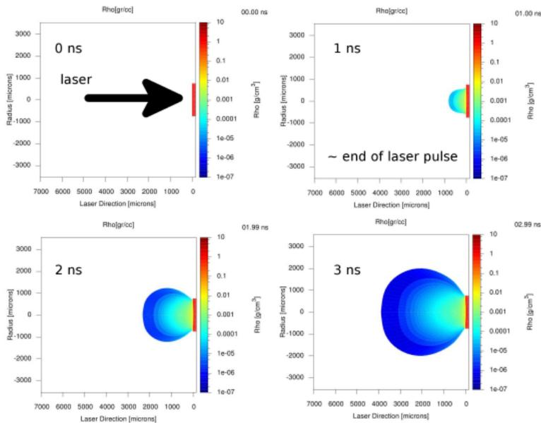
▷ Laser-target interaction with the 2D Lagrangian, radiation hydrodynamics code DUED (*Atzeni et al 2005*)
