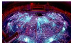
Z-machine in the USA has 11.4 MJ of stored energy and delivers a 20 MA current in 100 ns
