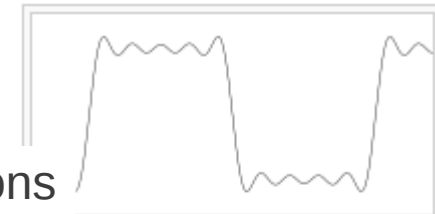
Functional approximation of square wave using 5 harmonics
