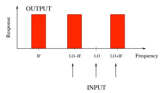
noise amplifiers and then passed through a filter which admits only one sideband (single-sideband mixer). Fow  $\nu \ge 100$  GHz, it is difficult to make low-noise amplifiers, so both sidebands are accepted for weak signals (double-sideband mixer).
